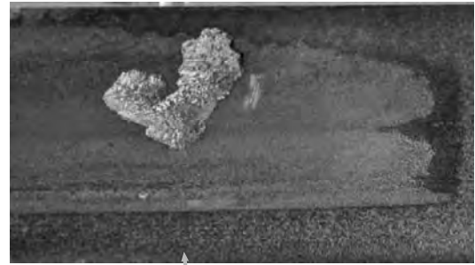
Fig.2 Trace of meshed-in foreign object and resulted flaking failure of hard tooth flank
