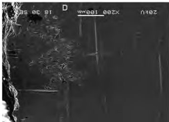
Fig.17 SEM figure of the surface near the broken position of the test piece (Position D). Surface damage due to crush of meshed-in foreign object
