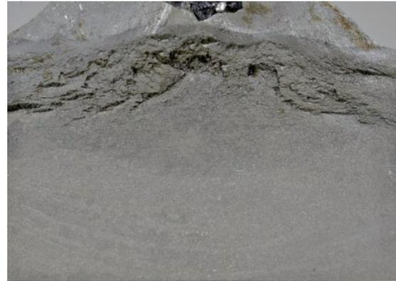
Fig.22 Propagation of micro-crack and it grows to be macro-crack to make fatigue breakage
