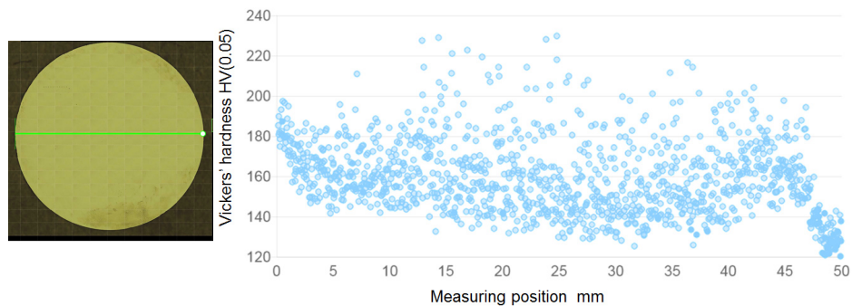
Fig.2 Result of non-uniform roll-pressing at production of SCM415 steel bar from the billet
