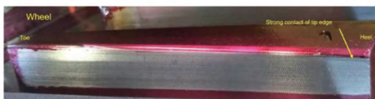
Fig.8 State of tooth flanks after 9hrs run
