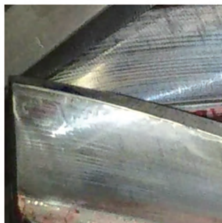
Fig.10 Soft contacting state of tooth flank near toe
