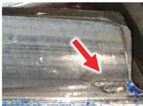
Fig.9 Peeling-off spot of pinion dedendum (severest spot)
